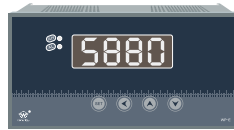
外形尺寸:160×80×125mm 开孔尺寸:152 +1 ×76 +1 mm
