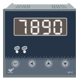
外形尺寸:96×96×76mm 开孔尺寸:92 +1 ×92 +1 mm
